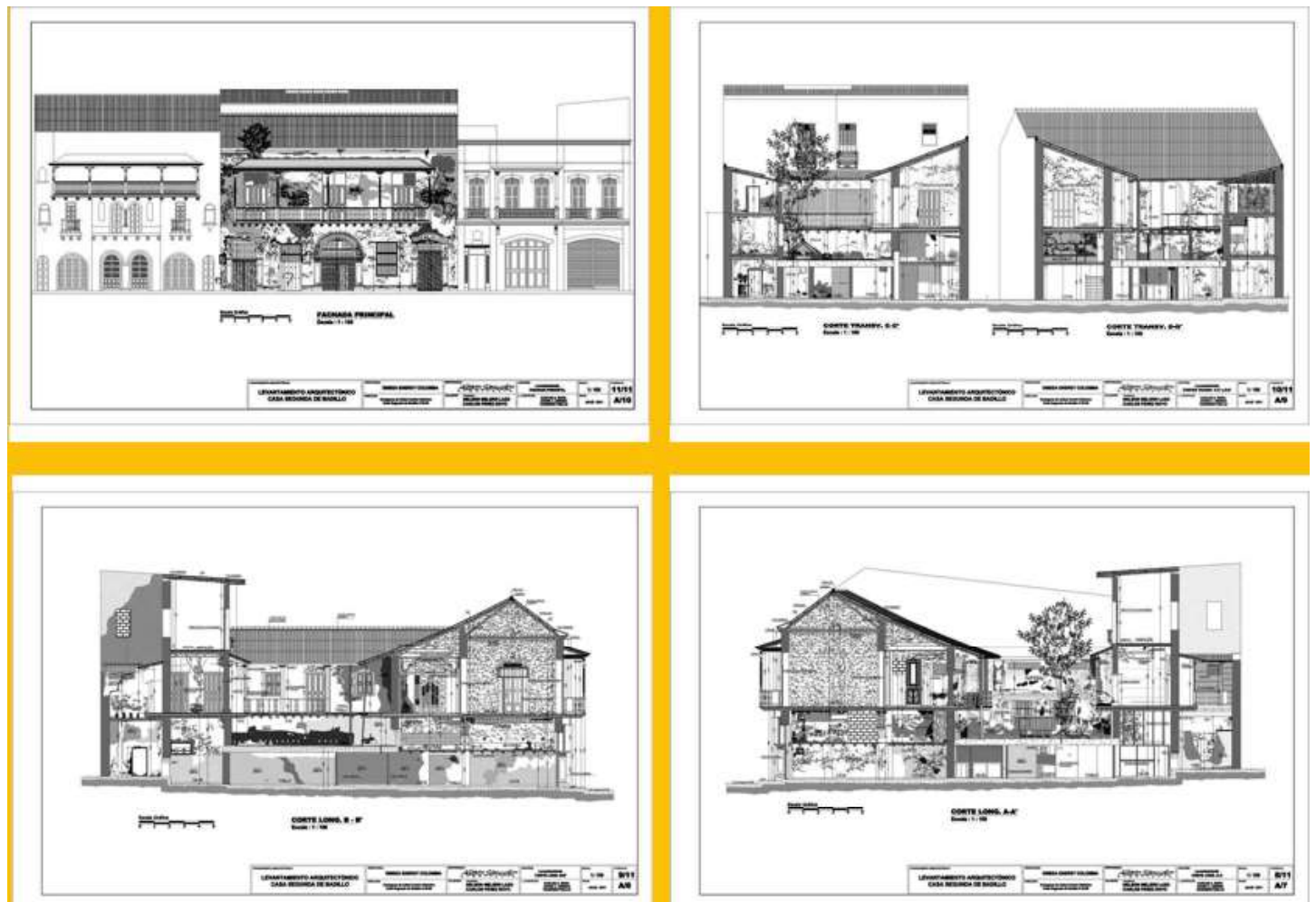
Figure 5. Plans Planes Surveying. Graphic representation with digital instruments. Palacio de la Proclamación. Cartagena de Indias. Colombia. Source: Melero, 2013.
